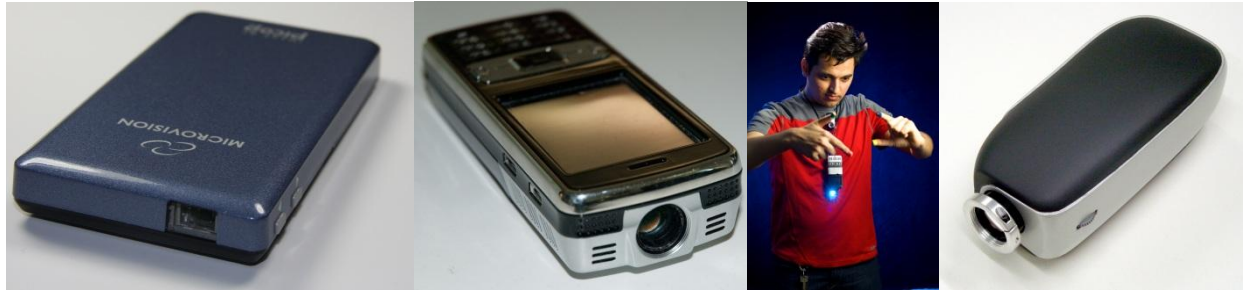
Figure 1. Personal projector concepts (from left to right): a. peripheral (Microvision SHOWWX), b. handset-integrated (Samsung W9600), c. wearable (figure courtesy of Pranav Mistry and his colleagues, photo by Sam Ogden) and d. standalone (figure courtesy of Stefan Rapp and his colleagues)
